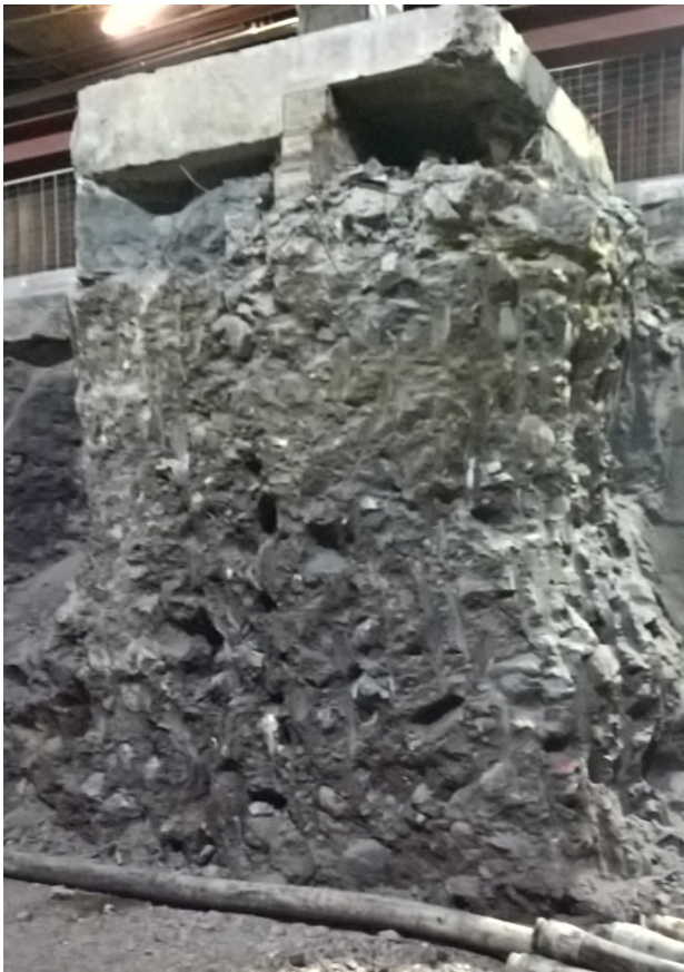
Figure 4 – Photograph showing undrained behaviour of the Glacial Till
